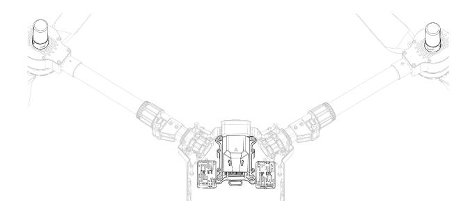
Please refer to the above picture to mount RTK mobile modules on the frame and make sure they do not vibrate.
