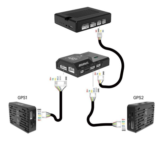
Please refer to the above picture and connect two F9P RTK mobile stations to the flight controller. The flight controller connects to the air unit of datalink.
