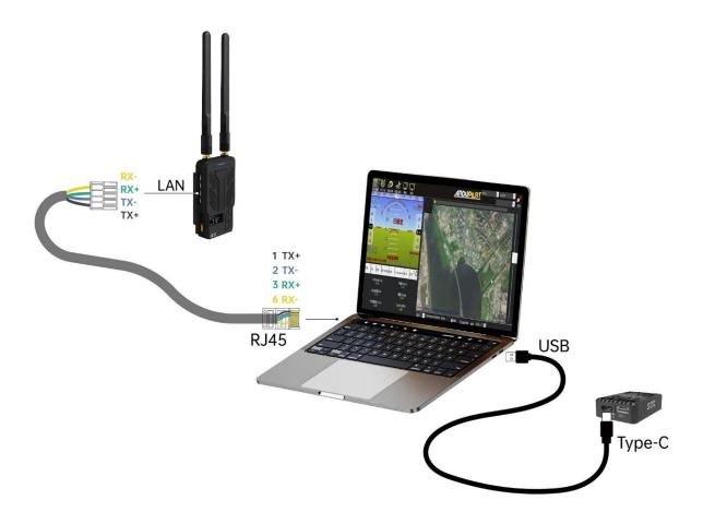
Please refer to the above picture and setup F9P RTK base station. The base station communicates to Windows GCS and sends real-time location of the RTK base station to flight controller.
