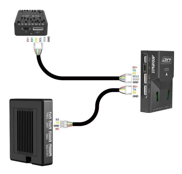
Please refer to the above picture and connect F9P RTK mobile station to the flight controller. The flight controller connects to the air unit of datalink.
